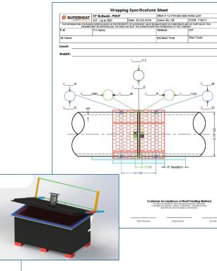
With DraftSight Professional software, Superheat not only can read in DWG files of customer products requiring heat treatment but can also manipulate drawing layers on heat-treatment designs to remove its sensitive IP from drawings or include it if clients choose to purchase drawings containing all layers as part of their heat-treatment solution.
