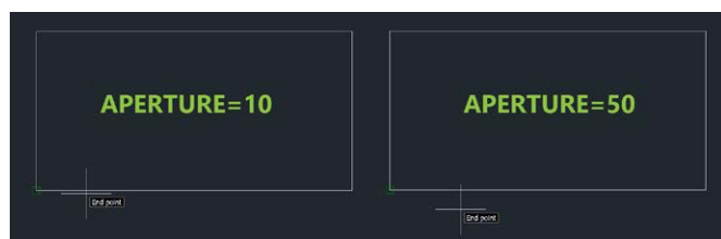
Figure 13. Aperture - the snap detection area around the cursor
